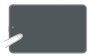
• On the **Control Panel**, press the **Power** key. If the Weekly Timer setting has put the machine in Erp Auto Power off mode, press the **Power** key to display the **Touch Panel**. To use it outside the preset operating hours, follow the on-screen instructions.
